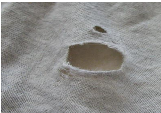
Unrepaired Hole 1" in any Dimension
